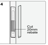
Place middle section of template into rebate and mark second rebate outline. Ensure it is the correct way up. Cut 20mm rebate
