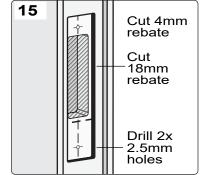
Place middle section of template into rebate and mark second rebate outline. Ensure it is the correct way up. Cut 18mm rebate
