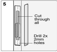
Mark the third rebate outline. Cut through into flush pull cavity.
