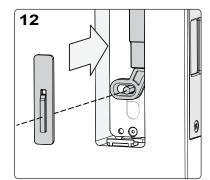
Insert emergency release onto the spindle.
